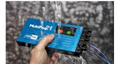
Data Logger Reset the data logger and connect the thermocouples to your product.
